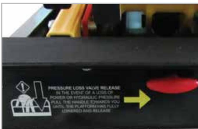
Emergency pressure loss valve release handle
