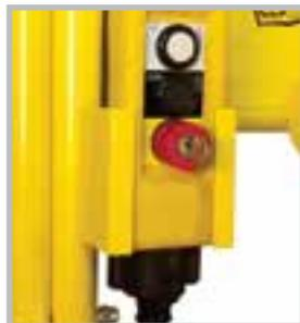
BoSS X-Series machines are fitted with an overload sensor system. If the platform load is exceeded the platform will not raise and the red LED indicator on top of the handset will illuminate as shown on the right.
