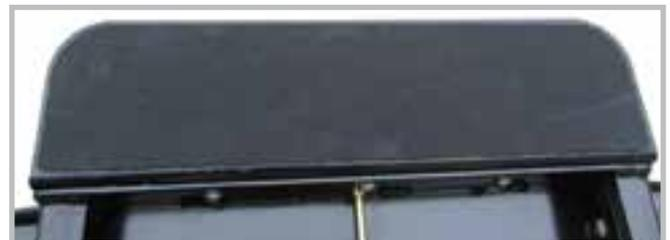
The stowed length of the BoSS X3X is reduced from 1.41 to 1.3 metres when the step is removed.
