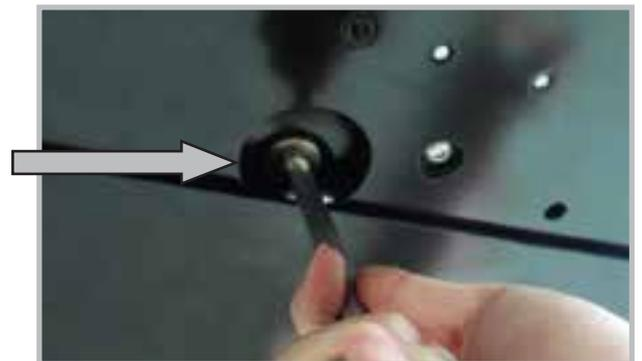
6. Undo the bolt and let the oil drain into an open top container which can hold a minimum of 2 litres. Dispose of the oil at an approved disposal facility.
